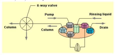
Post-injection rinsing function Rinsing liquid can be chosen from any positions. Syringe, needle, injection port, and injection valve are rinsed.
