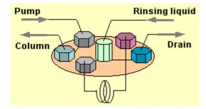
System configuration with double-injection rinsing function
